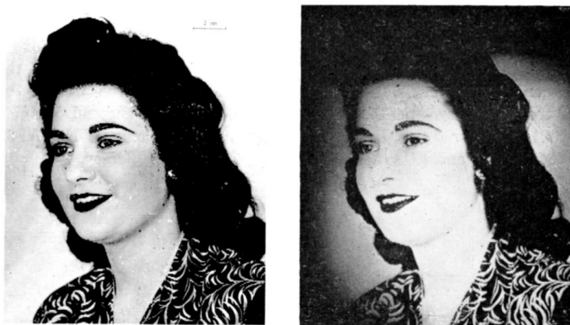
Fig. 6—Original and projected thermoplastic image. On the left is an enlargement from the photographic screened negative master and on the right is a rephotograph of the projected thermoplastic image ( 2 \times 3 feet) made from that master.
